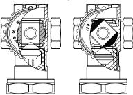
Versatility of the wall mounting bracket: the universal bracket 42D.DN25 (accessory) makes it possible to install the group with flow upward, downward or with the group laying on a side. Pay however the maximun attention to correctly fix the group to the wall when installed laying on a side.
