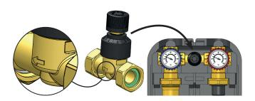
**Heat metering:** 23G.DN25 groups are equipped with specific extension to install energy metering devices, G 3/4 110 mm or G 1 130 mm. They are also complete with pocket for immersion temperature probe on the red knob monobloc.
