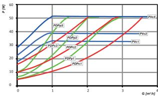
PVc: Power consumption at constant speed PDPp: Power consumption at proportional pressure PDPc: Power consumption at constant pressure
