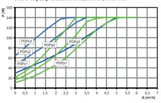
PDPp: Power consumption at proportional pressure PDPc: Power consumption at constant pressure
