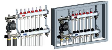
The group can be directly connected to a generator if the latter is not equipped with a pump. Instead, if the generator is equipped with a pump, an hydraulic separator should be placed between the generator and the group, in order to avoid mutual influences between the pumps. The group can be installed downstream of an inertial water storage, which performs the function of an hydraulic separator.
