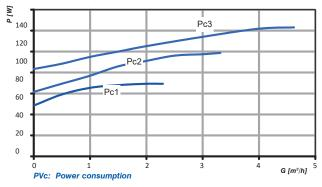
manifold and the 130 mm pump make the installation very compact. **Pump range:** the groups are available with three different pump models. For the use of other models and/or manufacturers, it is advisable to contact Barberi for verification.
