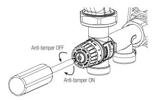
**FIRST SYSTEM START UP.** The fixed point temperature value can be set with the knob before installing the group or, after the installation, exclusively with the SYSTEM COLD. To set a temperature value different from the factory one, proceed as follows:
