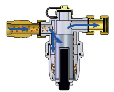
Fig. B: decantation and mechanical filtration
